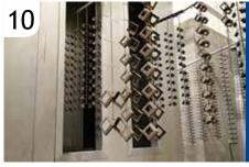
The powder coating is then bonded and adhered to the aluminum sub-straight in a 400 degree cure stage.
