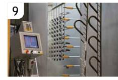
Powder is applied with 18 automated and 2 manual spray guns. Compressed process air is dried to -35°F Dew Point for superior adhesion.
